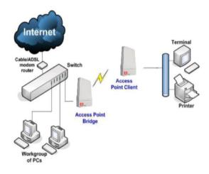
In the example above, the workgroup PCs will be able to access the printer connected to the access point in **Access Point Client** mode.
