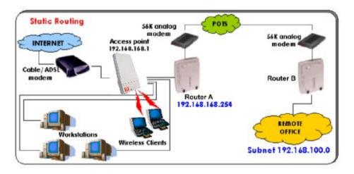
In this network, the main office of subnet 192.168.168.0 contains two routers: the office is connected to the Internet via the access point (192.168.168.1) and to the remote office via NetPassage 16A (192.168.168.254). The remote office resides on a subnet 192.168.100.0.
