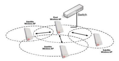
Here, the root Wireless AP connects to the wired network and maintains three WDS links while each satellite Wireless AP (Access Point) maintain a WDS link for communication with the root.
